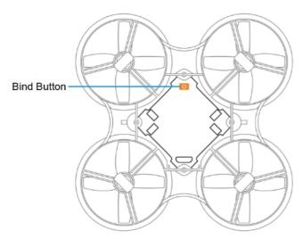
DO NOT press and hold the button before inserting the battery. It will erase the firmware and need to re-flash the firmware according to the manual above.
