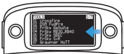
Push the right 5-D button to the left for 1 second to enter the tool setting mode
