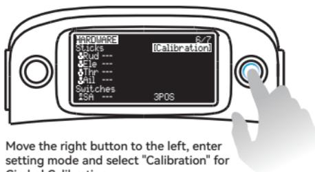
Move the right button to the left, enter setting mode and select "Calibration" for Gimbal Calibration
