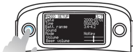
Short press the left side 5-D button to exit the setting mode and return to the default interface
