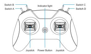
The top of the LiteRadio 2 SIM remote controller is as shown below.
