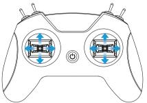
• Short-press the power button again, and the remote controller will record the boundary of the joystick and complete the calibration.
