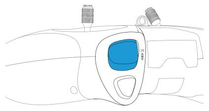
Move the Switch SC Up and Down to Change the Speed Threshold
