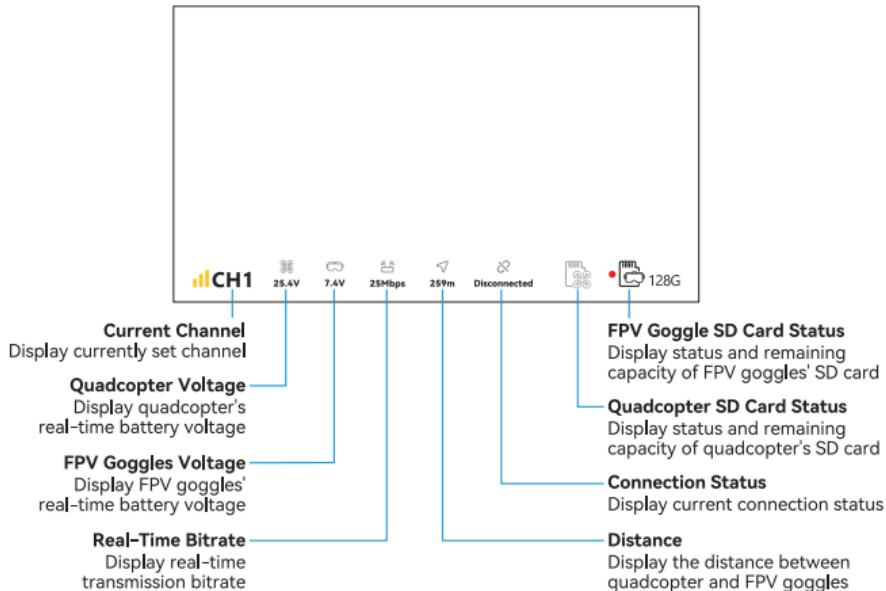
Note: SD card status: gray light is displayed when no SD card is inserted, bright color is displayed when an SD card is inserted, a red dot flashes when recording, no red dot is displayed when not recording, and Full is displayed when the card is full.
