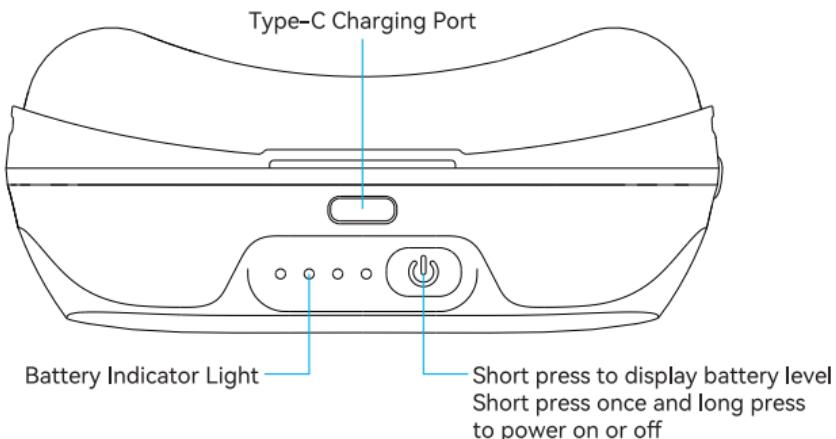
Note: When only left one battery indicator light flashes, recharge the battery timely to prevent the goggles screen from turning off due to low power.
