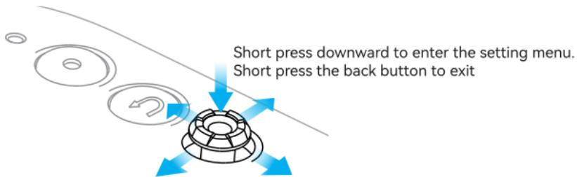
On the main interface, short press the 5D button will open the menu. The 5D button can be used to select menu items by going up, down, left, and right. Pressing the back button will return to the previous menu.
