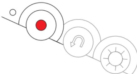
Short press to start recording, short press again to stop recording and save
